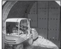
Bricks being stacked in kiln for firing
